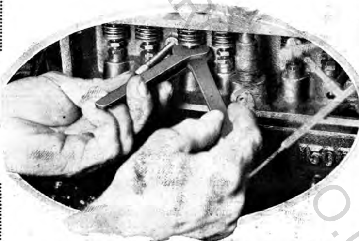
Tightening up the tappets after setting. The tappet stem and tappet screw should be held in position by the special tappet spanners while the tappet lock nut is firmly tightened with the appropriate double-ended spanner from the tool kit.
