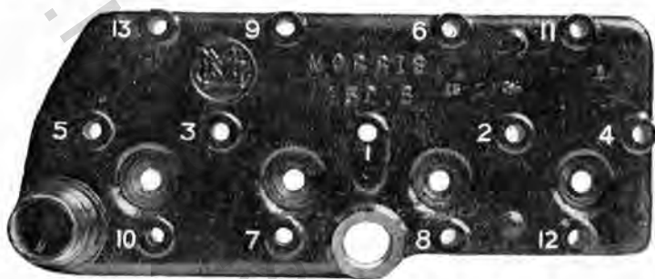
Indicating the sequence in which the cylinder head stud nuts should gradually be tightened.
