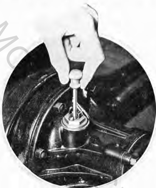
The oil filling plug of the Morris Eight rear axle, which also serves to indicate the oil level by means of a dip-stick.
