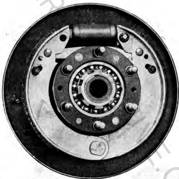
The brake-drum removed, showing the rear brake-shoe assembly. The assembly for the front shoes is identical, with the exception of the hand-operating mechanism.
