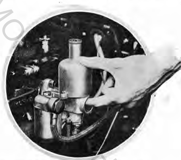
By inserting a finger in the air intake the piston may be raised or lowered to free its action.
