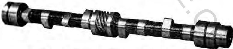
The camshaft is of generous dimensions and carried on three large bearings.
